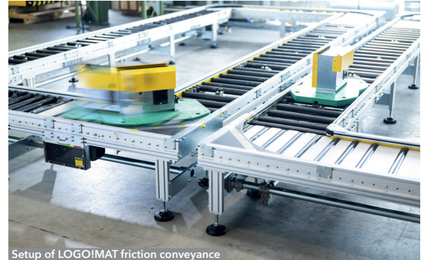
Setup of LOGO!MAT friction conveyance
