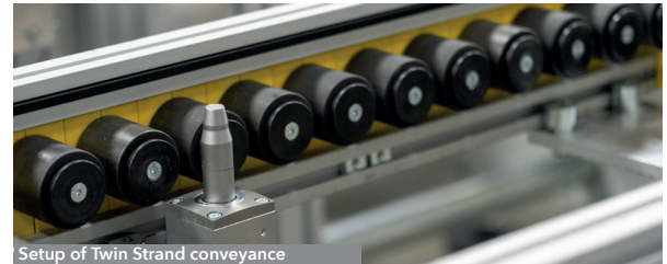
Setup of Twin Strand conveyance
