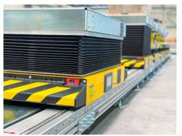
using the Scissor Lift. An eCart can approach and position itself beneath the part, raise its Scissor Lift to index into it, and carry the part along to the next station.
