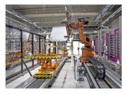
The eCart's passive track system contains no moving parts and is totally maintenance-free and completely accessible; operators can safely step on and around the entire track to access all sides of the part. This saves considerable investment and operating costs in regards to the interlinking of assembly modules when compared to traditional conveyor systems. This also applies to the adaptability of the system when it comes to increasing or changing demands from the end
