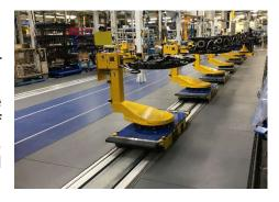
The eCart system takes over part transportation in automated assembly lines for chassis (e.g. front and rear axles), interior (e.g. seats, cockpits) and exterior (e.g. frontends) components, Just in Sequence. The efficiency and intelligence of the eCart system enables the production and delivery of vehicle modules at the exact time, place, and in the order they are required for final assembly.
